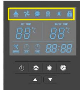
**IMPORTANT:** If the fan is active without the heating symbol, you may have activated the ventilation mode. This should only be used with properties with air conditioning features enabled.
