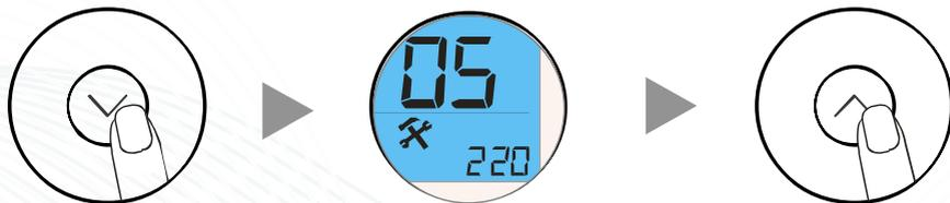
Use the up button to move through the parameters
