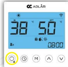
**\*IMPORTANT:** It is not necessary to turn off the heat pump. The dynamic heating curve control ensures that the heat pump never switches on when the set room temperature is lower than the desired temperature.
