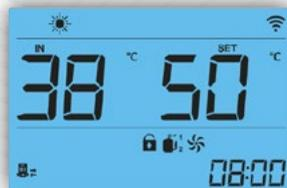
**IMPORTANT:** The symbols indicate operating modes. They are not permanently shown, and will change based on the operation state of the heat pump. If the set water is close to the inlet/outlet temperature then then symbols should turn off as the heat pump modulates.
