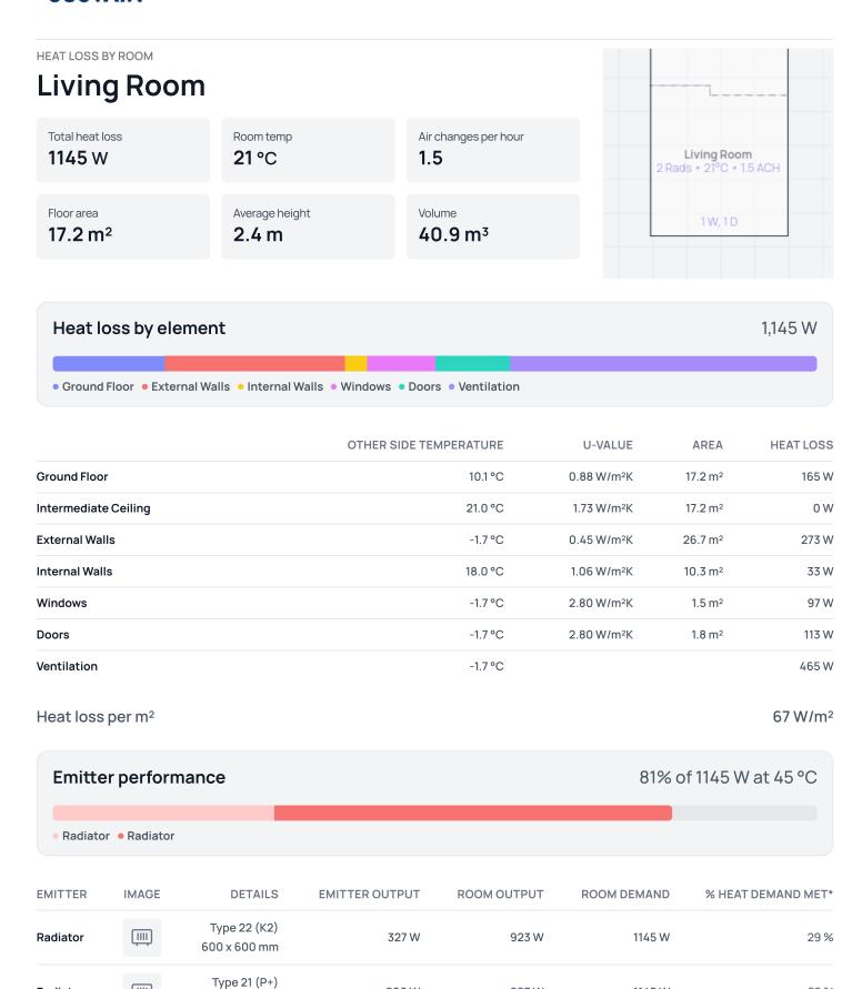
$<sup>\</sup>textbf{*\% Heat demand met:} \ \text{This is calculated for a day when the outdoor temperature is -1.7 °C} \ \text{and the flow temperature is 45 °C} \ \text{This is calculated for a day when the outdoor temperature} \ \text{and the flow temperature} \ \text{and the flo$
