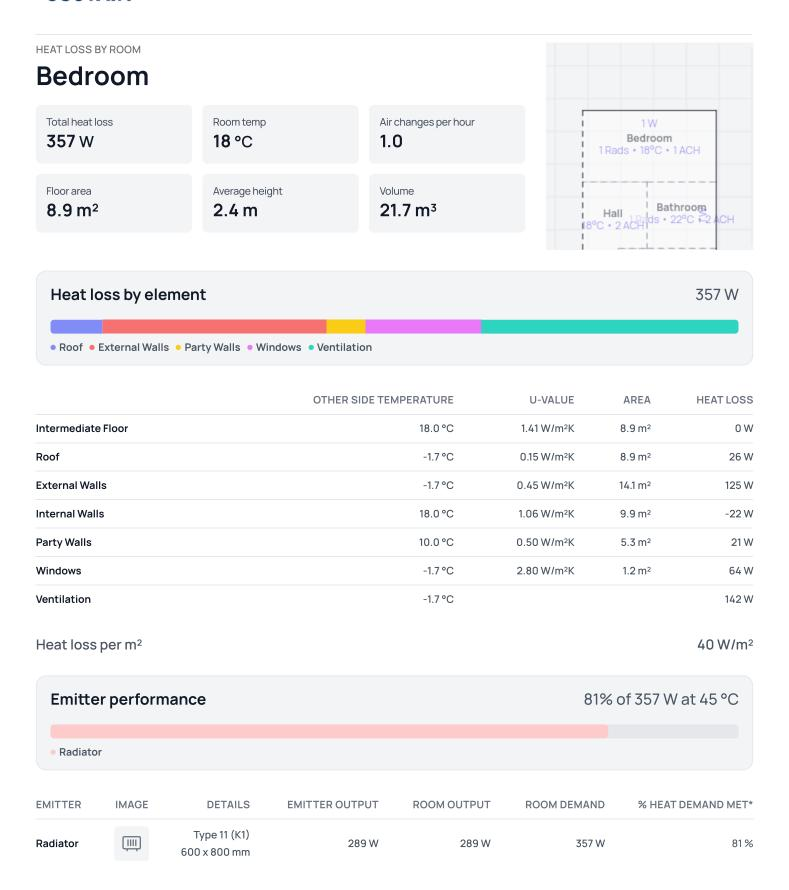
$<sup>\</sup>textbf{*\% Heat demand met} : \textbf{This is calculated for a day when the outdoor temperature is -1.7 °C and the flow temperature is 45 °C and the flo$
