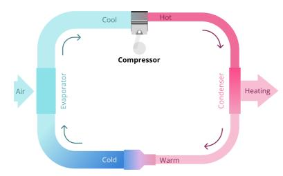
The beauty of heat pumps is that a relatively small electricallydriven compressor can move large amounts of heat. The ratio between the electrical energy input and the heat output is the coefficient of performance (CoP). This will vary over the course of a year: the heat pump will be more efficient in the summer when the difference between the inside and outside temperatures is less.
