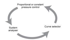
Fig. 29 The AUTO<sub>ADAPT</sub> three-step task
