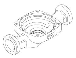
Fig. 49 Pump housing
