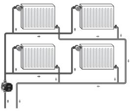
Fig. 3 Two-pipe heating system
