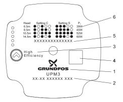
Fig. 6 Nameplate: Grundfos with setting indication
