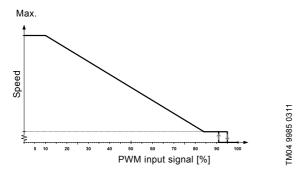
Fig. 14 PWM input profile A (heating)
