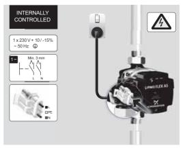
Fig. 64 Control box without signal connection
