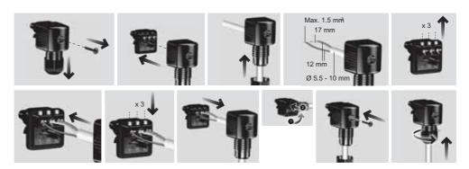
Fig. 67 Superseal installation plug
