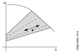
Fig. 34 New lower proportional pressure curve
