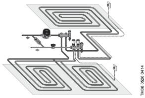
Fig. 4 Underfloor heating system
