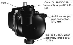
CIAO2 AC composite, inline, air outlet, alternate connection
