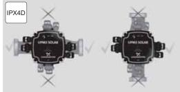
Fig. 53 Control box positions
