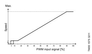
Fig. 15 PWM input profile C (solar)
