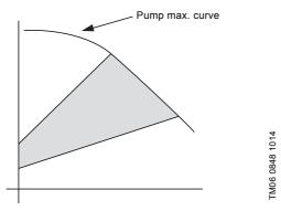
Fig. 30 Proportional pressure AUTO<sub>ADAPT</sub> operation area
