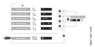
The pump automatically enables the PWM input-signal control mode by SignalDetect, when the signal cable is plugged in.
