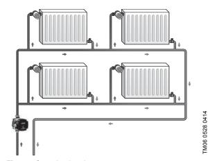
Fig. 2 One-pipe heating system
