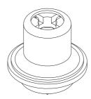
Fig. 40 Deblocking device
