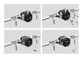
Fig. 54 Changing the control box position
