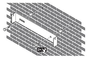
2 Hang the backup heater onto the wall bracket.
