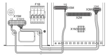
3 Fix the cable with cable ties to the cable tie mountings.
