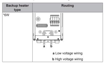
3 Fix the wiring with cable ties to the cable tie mountings.
