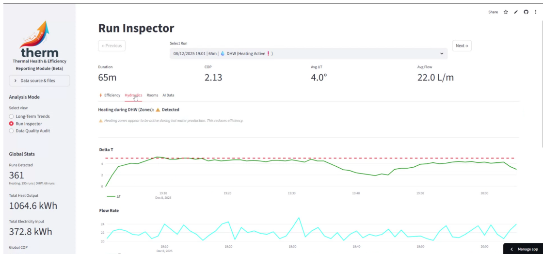
Figure 16 - DHW run with heating detected during DHW
