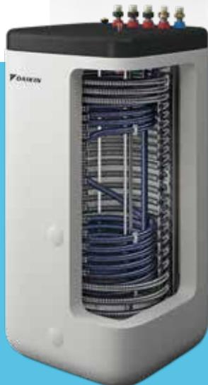
**Low scaling:** On commissioning, the storage tank is filled with tap water which is not exchanged during operation. Thus, only the lime contained in this water can be deposited; all the heat exchanger pipes remain free of limescale, as does the electric immersion heater, which is available as an option. On the inner surface of the heat exchanger pipes, the high flow speed when the water is removed releases smaller scale deposits.
