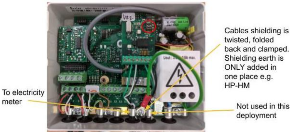
Sontex heat meter with RS485 module and mains supply
