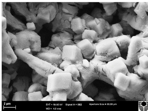
Fig. 11. High-magnification SEM images (scale bar: 2 μm) of scale formed in magnetized and non-magnetized tests of CSI-B.
