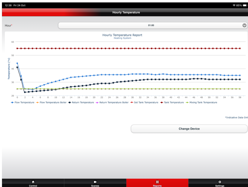
Figure 3 Mitsubishi MelCloud Report Flow Temperature, Return Temperature and Water Temperature 01.00-02.00
