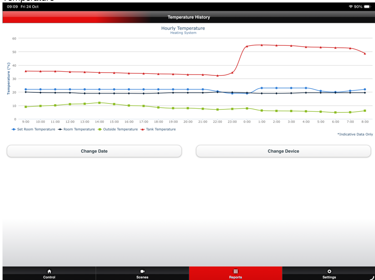
Figure 1 Mitsubishi MelCloud Report Outside Temperature, Room Temperature and Water Temperature
