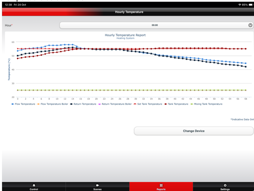
Figure 2 Mitsubishi MelCloud Report Flow Temperature, Return Temperature and Water Temperature 00.00-01.00
